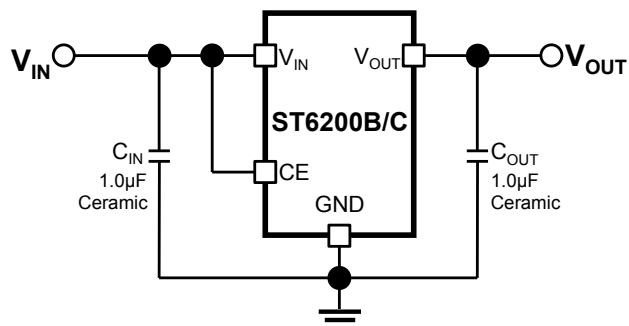
Figure 2: ST6200B/C Series Application Circuit
