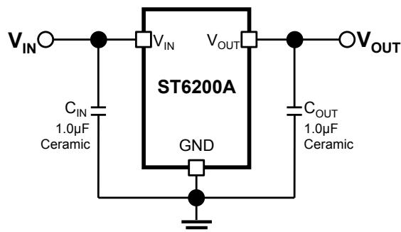
Figure 1: ST6200A Series Application Circuit
