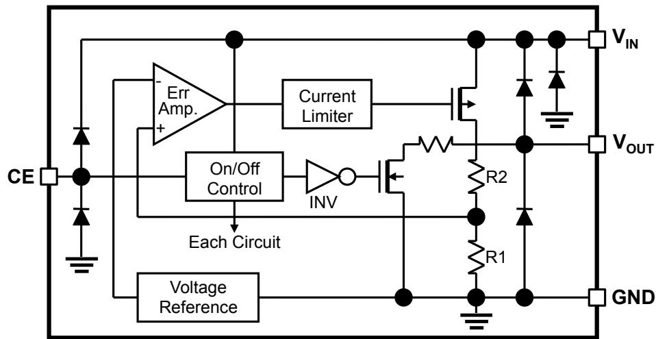
Figure 3: ST6200B Series Block Diagram
